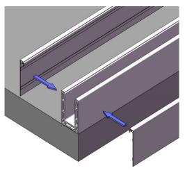
**Step 7.** Put the glass into aluminum channel.
