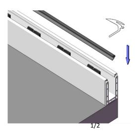
**Step 4.** Click side cladding on both sides of the aluminum channel.
