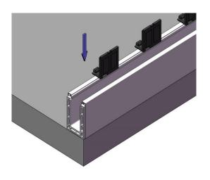
**Step 3.** Fix the aluminum channel on the ground.
