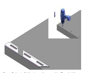
Step 5. Install the L wedge on the fixed side.
