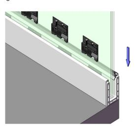
**Step 9.** Tighten the right bolt clockwise to adjust glass panel 1° to exterior (fall side). Tighten the left bolt clockwise to adjust glass panel 1° to interior
